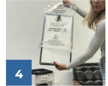
4 Remove plastic protectant covering from filters
